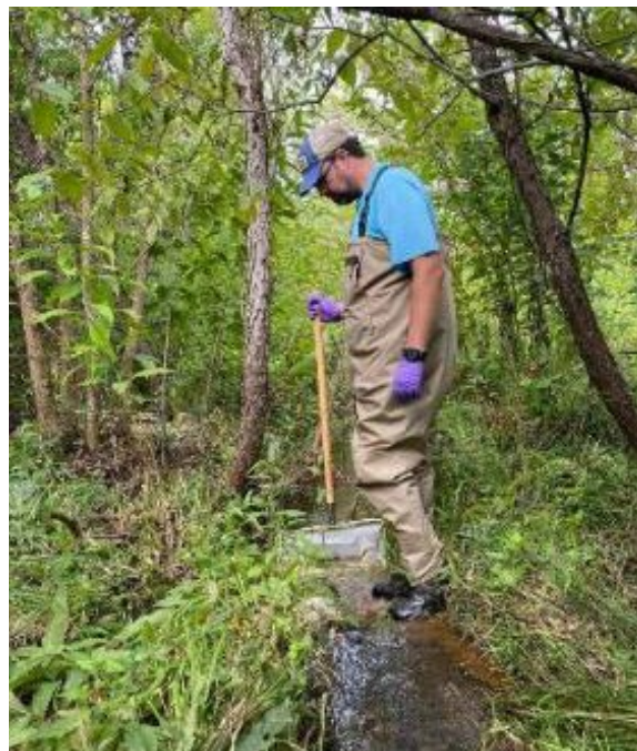
Figure 3.38. Sampling for benthic macroinvertebrates with TDEC protocols
